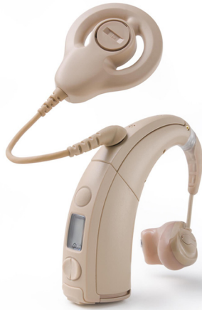
Figure 3. A hybrid sound processor from Cochlear Ltd. Intended for use by cochlear implant recipients with usable acoustic hearing in the implanted ear, this processor can control a CI to generate electric stimulation via the coil seen at the top of the picture, while acoustic signals are available simultaneously from the transducer seen at the lower right. Image provided by Cochlear Ltd.
