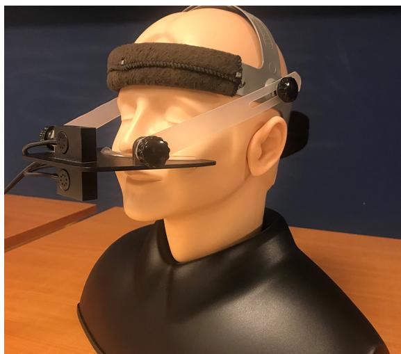
**Figure 1.** The Nasometer II device (Pentax Medical model 6450) used for nasal resonance imaging
